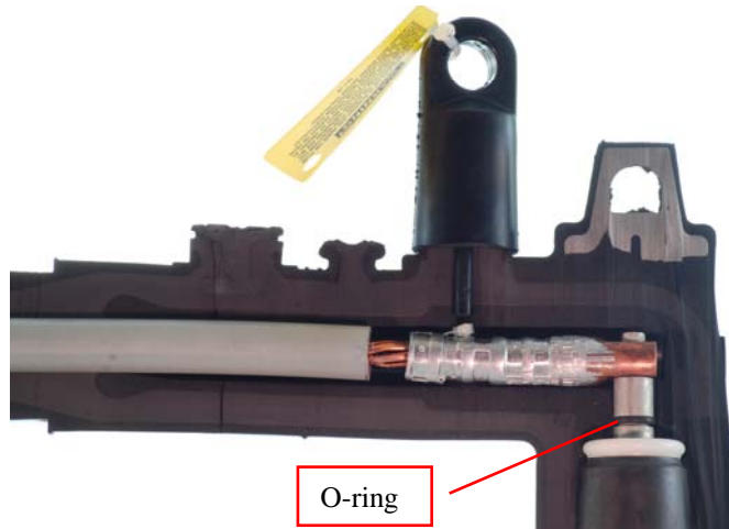
Figure 1. Cut-away of a typical injection elbow shows the placement of an O-ring just above the nose of the bushing.
