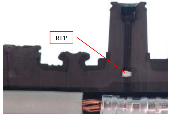
Figure 4. Direct access injection elbow used for unsustained pressure injection. The reticular flash preventer (RFP) is absent from older injection methods.
