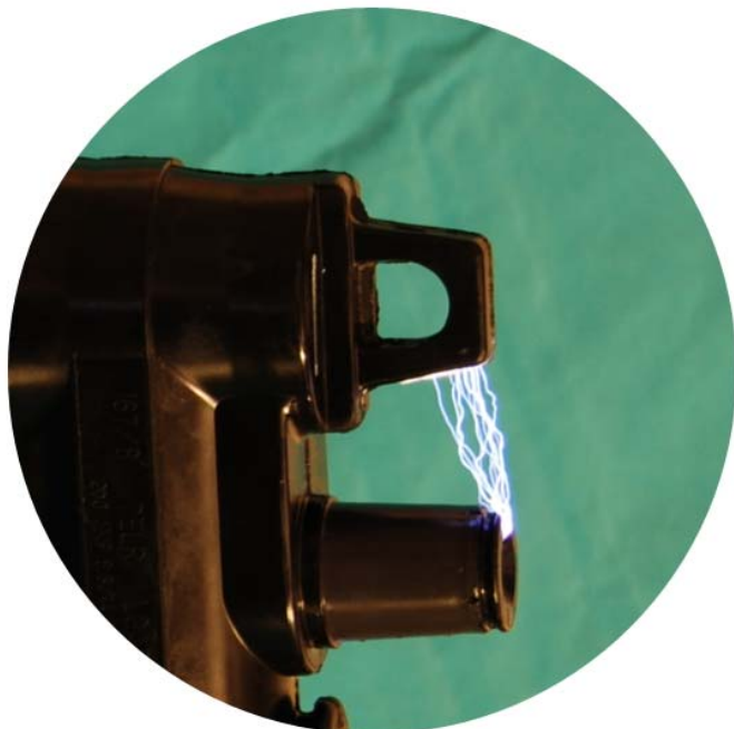
Figure 5. The relatively short distance of 3.5" from [14] for this 15kV injection elbow (4.7" for the 35kV large interface injection elbow of Figure 2) from the energized conductor to the nearest ground plane creates a flash hazard when the device does not have an RFP installed and the caps are swapped on an energized elbow. This laboratory photograph shows the initial current path.
