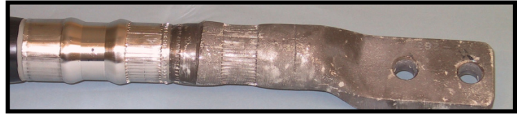
Figure 4. IA and lug swaged to cable.
