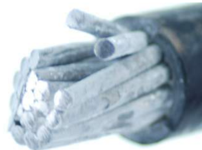
white powder is oxidized aluminum
